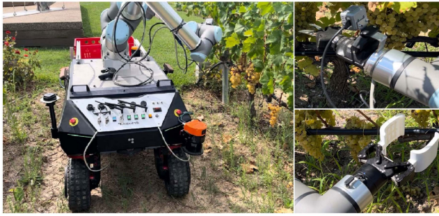
FIGURE 12. Heterogeneous end-effectors: using the bimanual control strategy [69].
