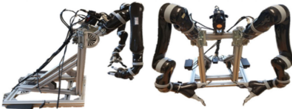
FIGURE 13. Homogeneous end-effectors: using the goal-coordinated control strategy [23].
