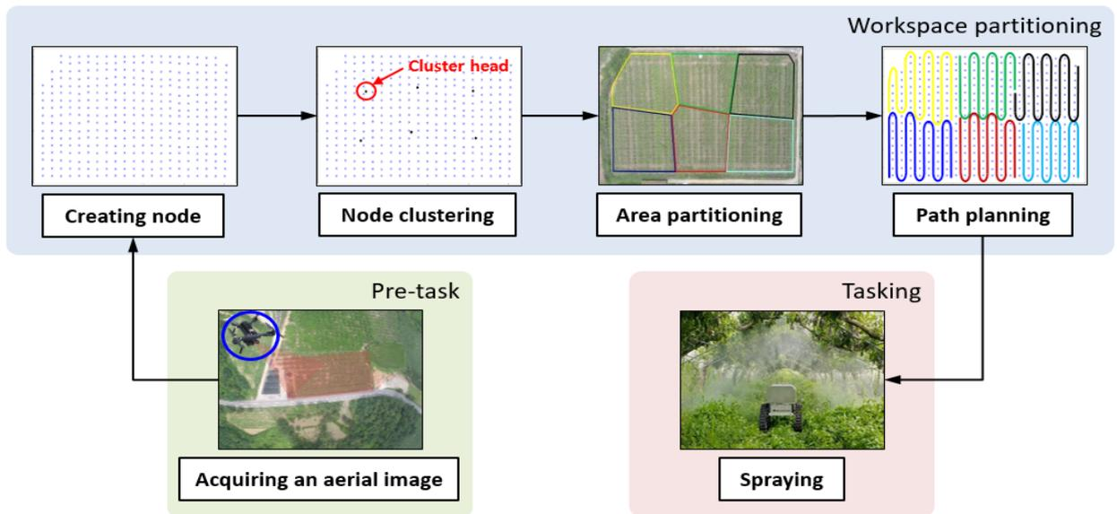
FIGURE 1. The global system flowchart of MRTA for spraying task.
